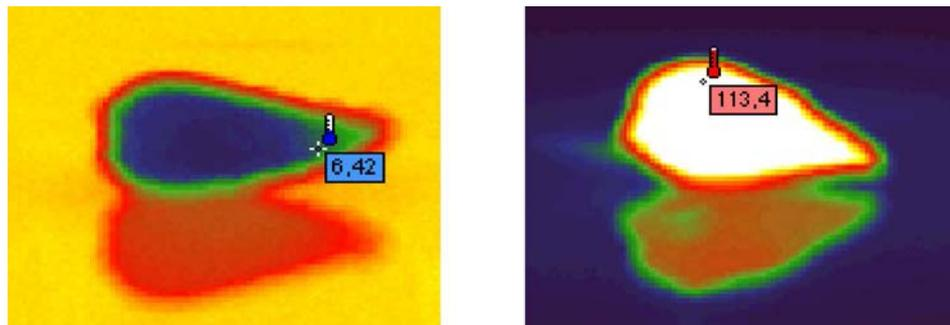
**Figure 5.** Example of picture cones heated by electromagnetic radiation 620 a – before, b – after 20 s
