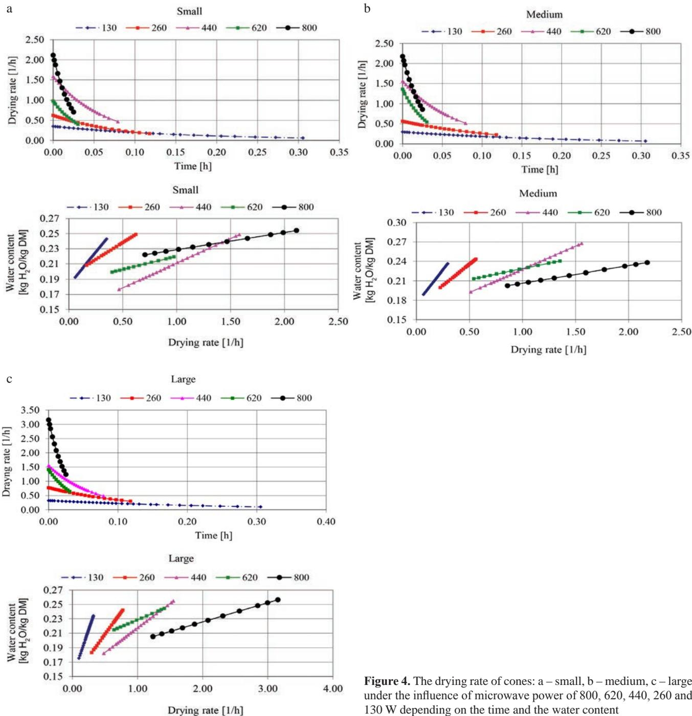
**Figure 4.** The drying rate of cones: a – small, b – medium, c – large under the influence of microwave power of 800, 620, 440, 260 and 130 W depending on the time and the water content
