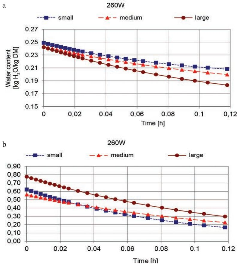
**Figure 3.** The changes in cones of small, medium and large size under the influence of microwave radiation with a power of 260 W, in terms of: a – water content, b – drying rate
