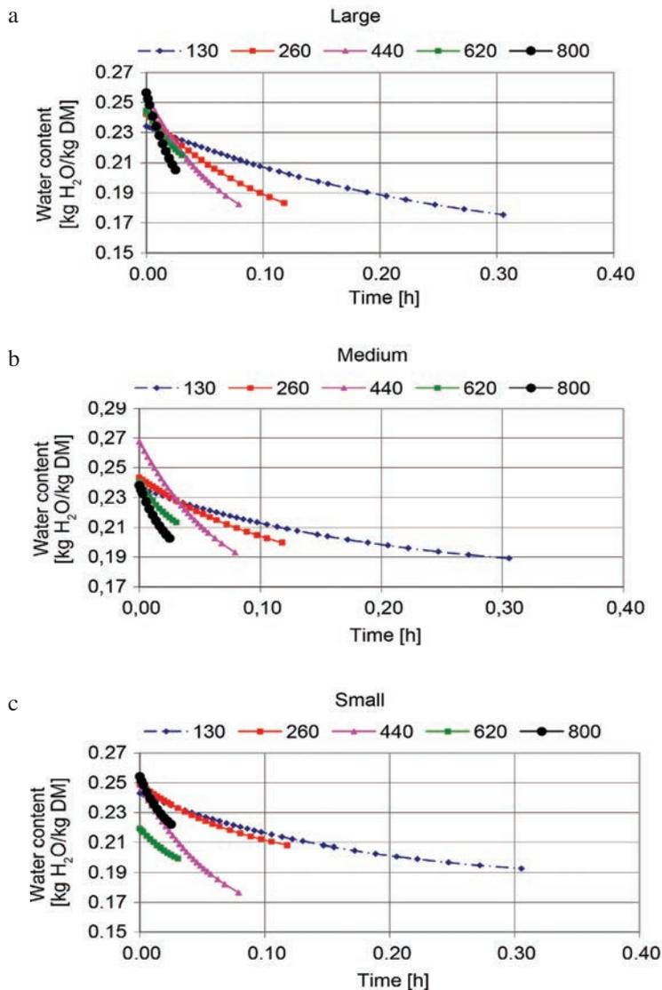
**Figure 2.** Change of water content in the cones: a – large, b – c medium – small under the influence of microwave radiation power: 800, 620, 440, 260 and 130
