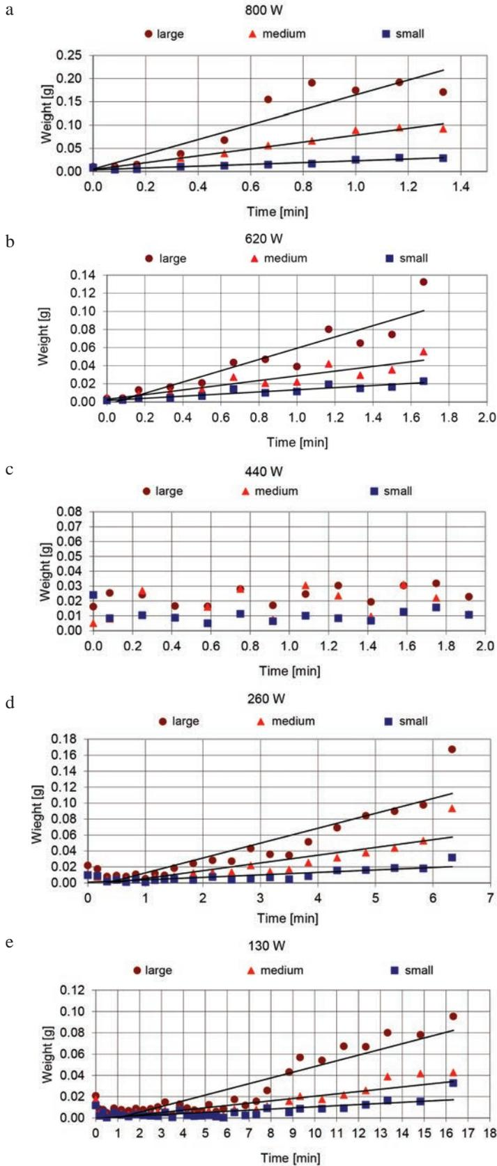
**Figure 1.** Weight change of small, medium and large cones under the influence of radiation-microwave with different power: a – 800 W, b – 620 W, c – 440 W, d – 260 W, e – 130 W
