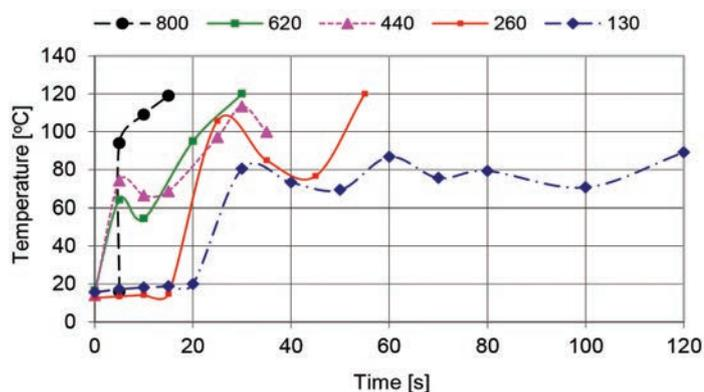
**Figure 6.** Changes of the maximum surface temperature of cones under the influence of microwave radiation
