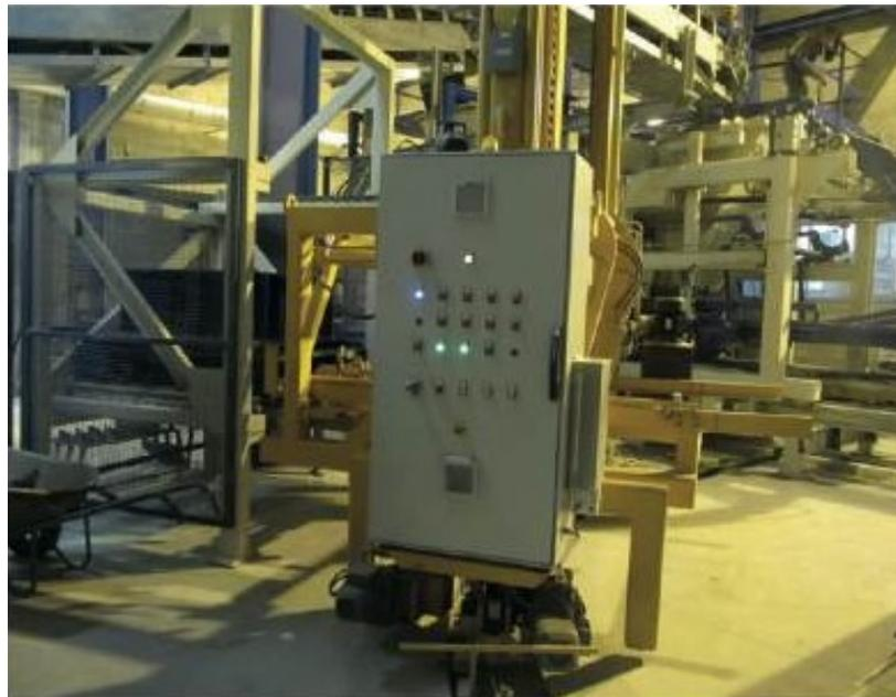
**Figure 2.** Stacker crane ready to incorporate the new mold [3].
