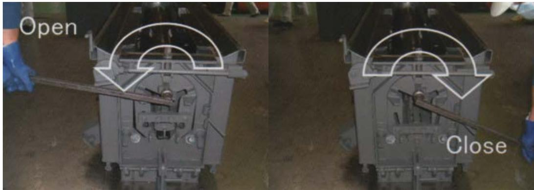
Figure 7. Opening and closing of inner in one-touch by hand [10].
