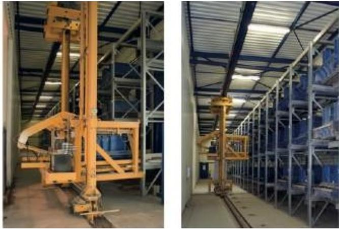
**Figure 1.** Automated mold rack storage [3].
